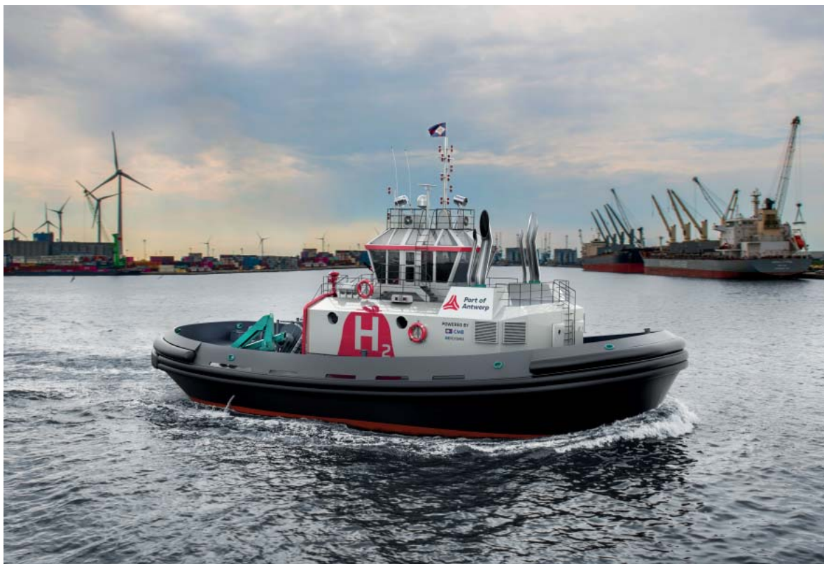
■ A rendering of the 65-tonne bollard pull Hydrocat, which will be powered by 2.6MW, V12 BEH2YDRO engines burning up to 85% hydrogen in combination with 15% diesel.
