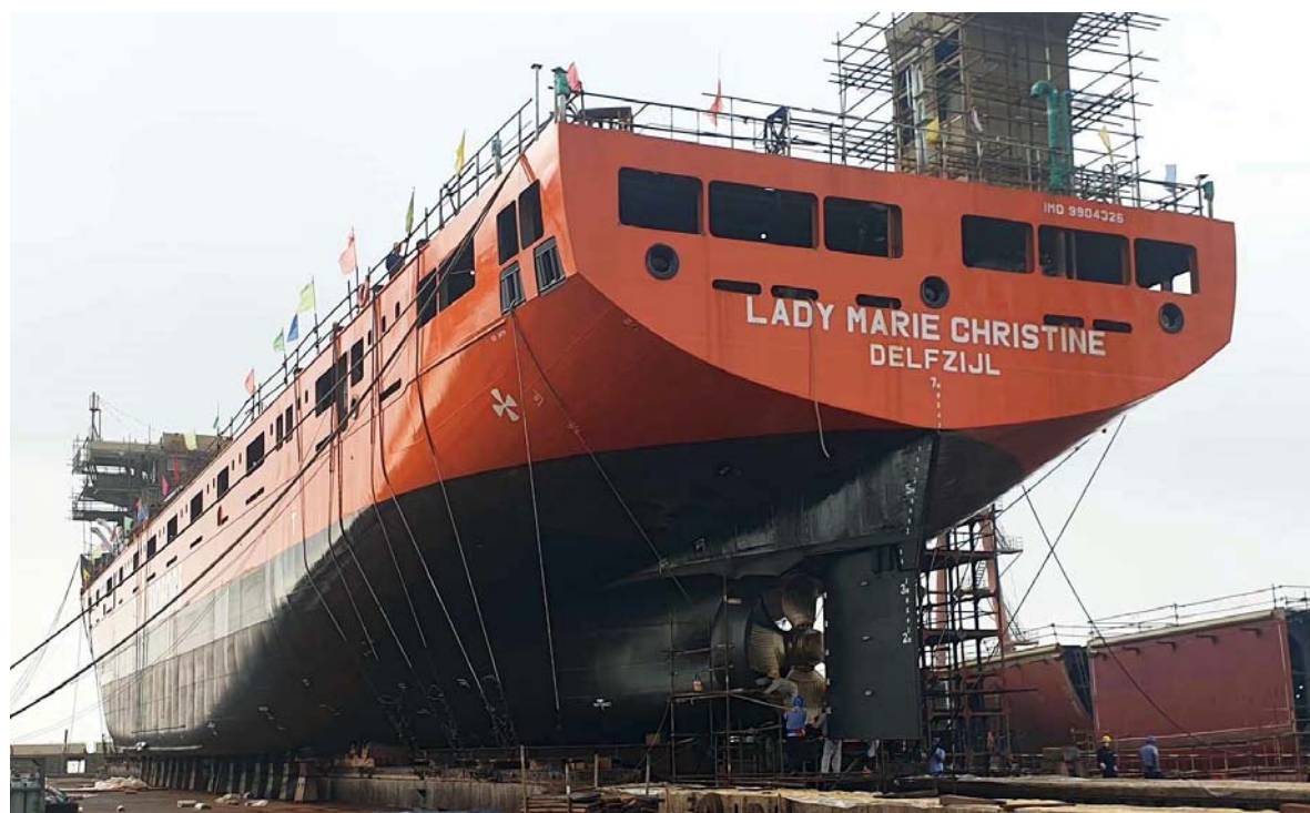
■ The hull shape of the new LNG-fuelled Lady M series was optimised by Conoship using CFD calculations
