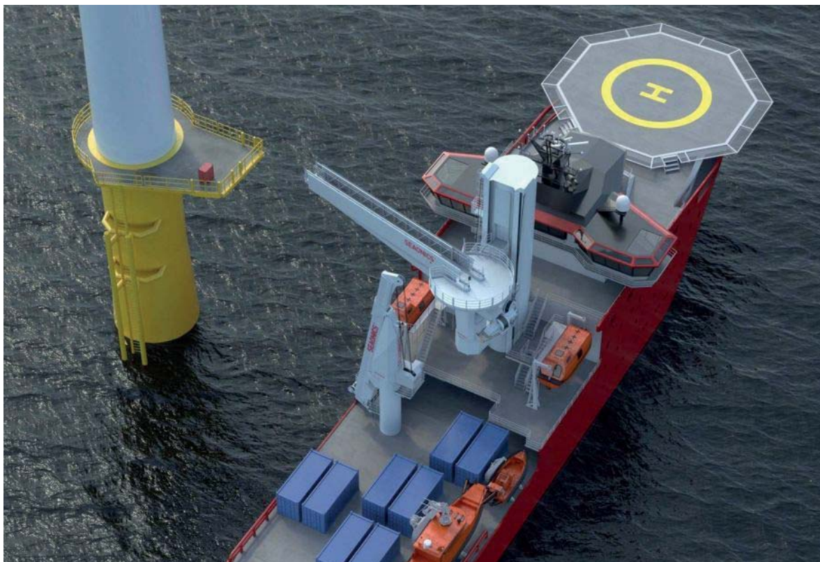
■ Palfinger's OPTS system is a multifunctional hydraulic aerial lift for transporting both people and materials in a safe, quick, and efficient way
